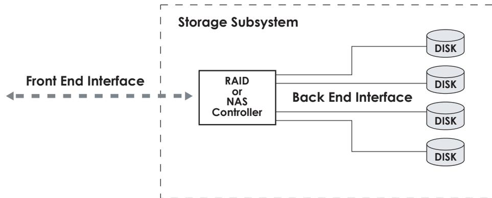
Front End interfaces such as 100/1000 BaseT Ethernet, SCSI or Fibre Channel provide storage-to-server interconnectivity within the data center. Connectivity between data centers within a campus (<10,000 meters) is sometimes done with Long Wave Fibre Channel over dedicated Fibre. Data centers that do not reside within a campus but are <80,000 meters apart may also take advantage of leased dark Fibre lines for a high price.
