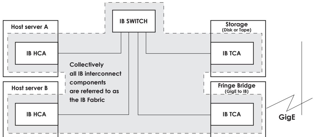
HCA technology is beginning to appear in the form of a PCI or PCIX daughter card that is inserted into a host server's existing I/O bus, similar to how one would install a Fibre Channel Host Bus Adapter or GigE NIC card.
