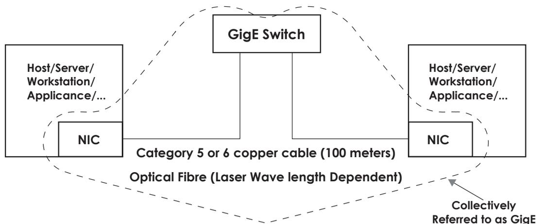
**NIC** – Network Interface Card – Provides the hardware bridge between the host's native bus and the 100/1000 Base-T Ethernet serial interface. Current low end (<\$300) GigE NICs rely heavily on the host system's CPU to perform TCP/IP stack processing. This limits throughput to <40 MB/second and fully consumes a 1 GHz Pentium 3. Second generation GigE NICs will take advantage of TOE (TCP Off-load Engine) technology and improve sustainable throughput in to the 80-90 MB/second range.
