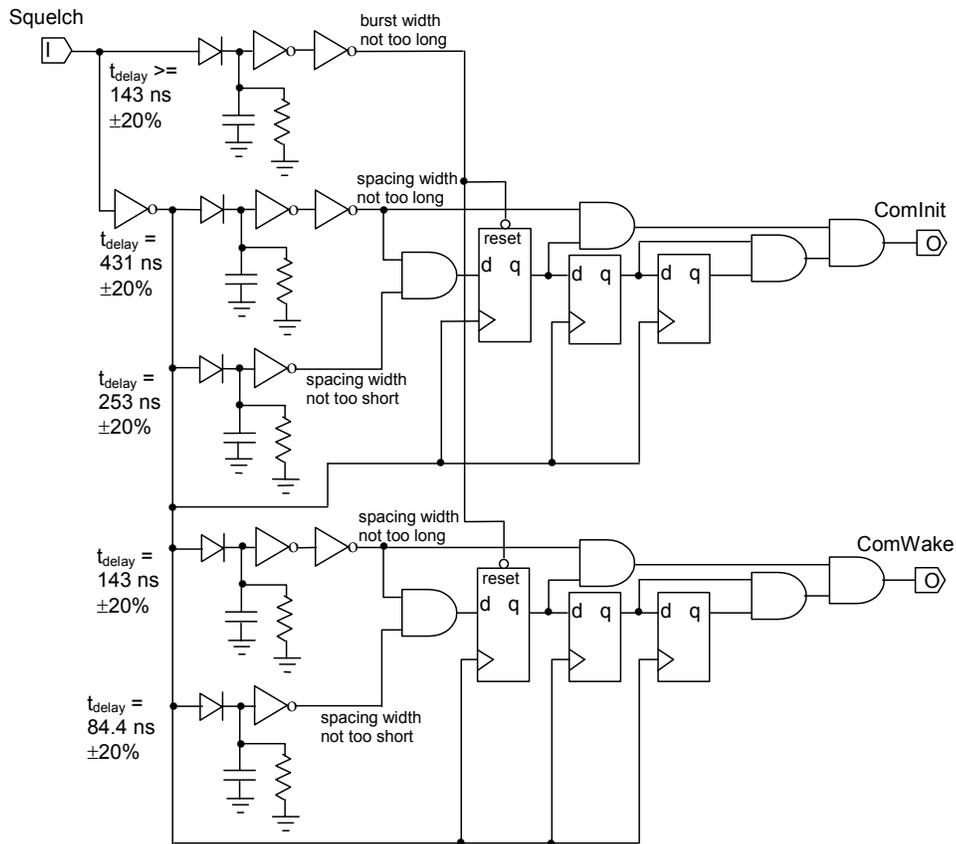
**Figure 32 – OOB signal detector**
