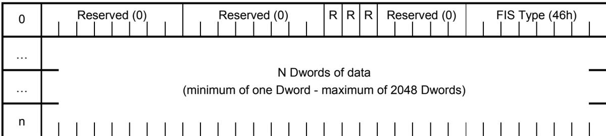
**Figure 66 – Data – Host to Device or Device to Host FIS layout**
