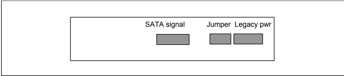
**Figure 70 - Device connector configuration 35B2**
