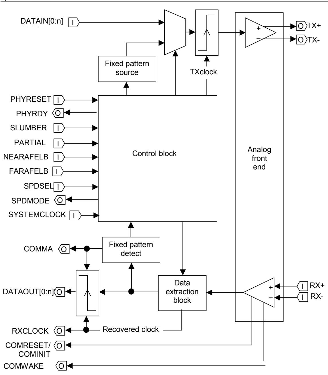
Figure 18 – Physical plant overall block diagram
