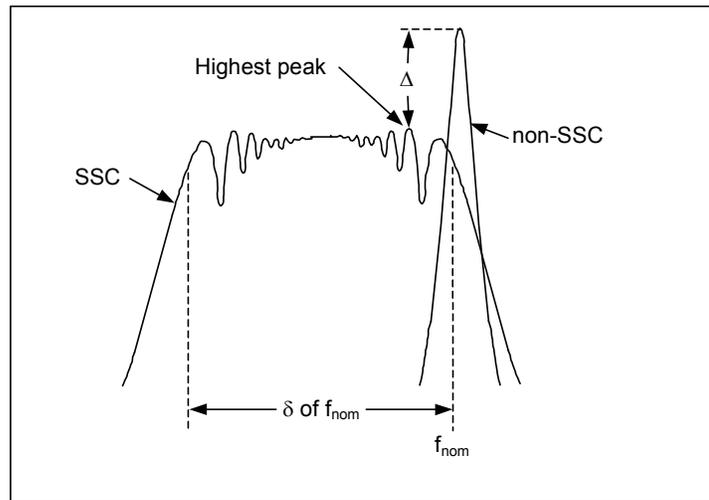
**Figure 26 - Spectral fundamental frequency comparison**
