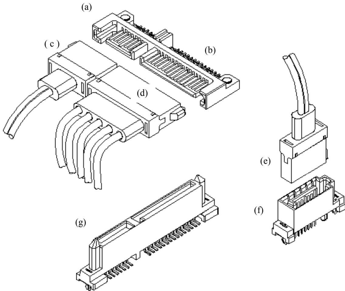
**Figure 5 – Serial ATA connector examples**
