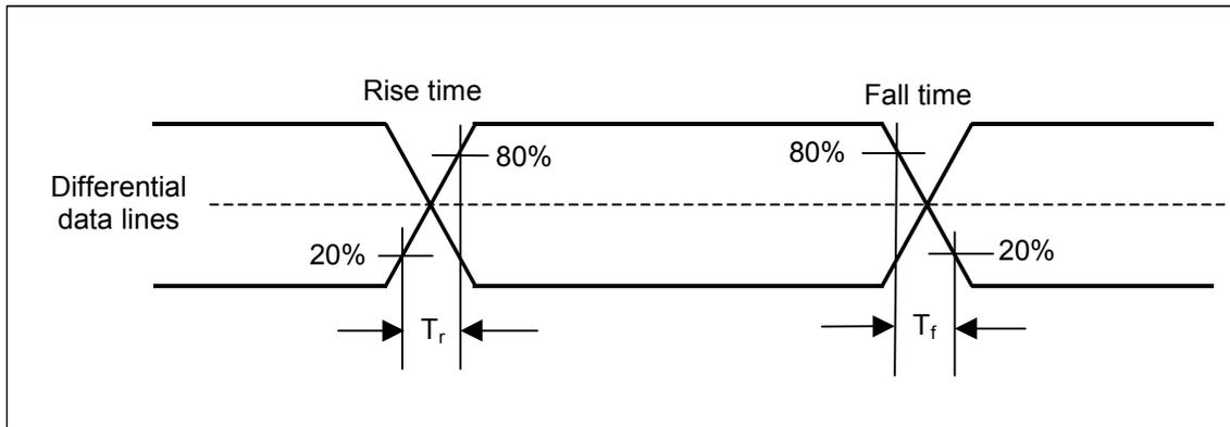
**Figure 44 – Signal rise and fall times**
