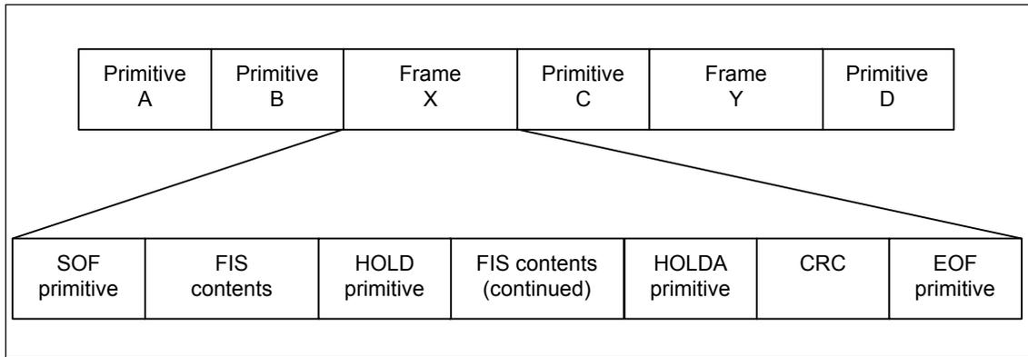
**Figure 57 – Transmission structures**
