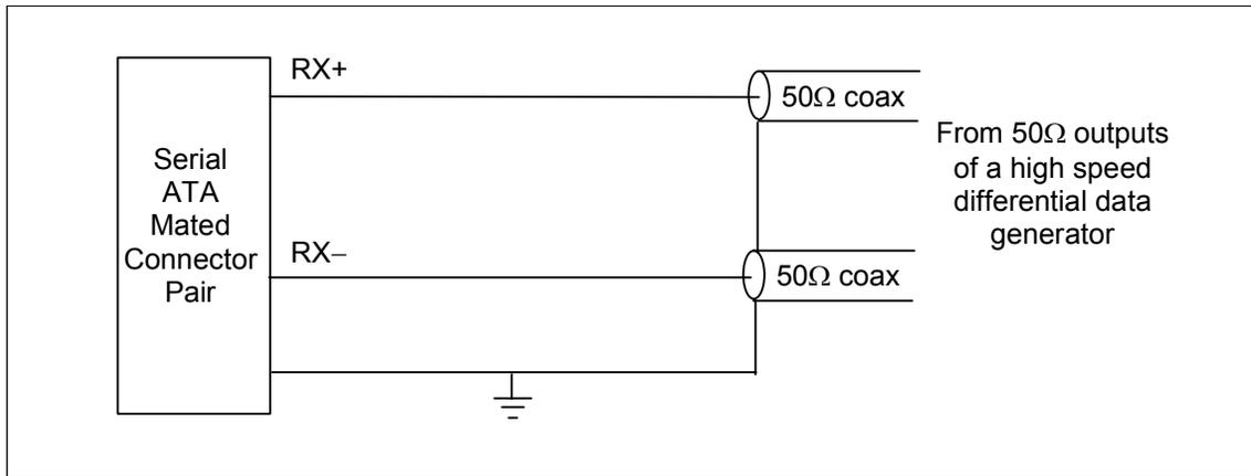
**Figure 46 – Receive test fixture**
