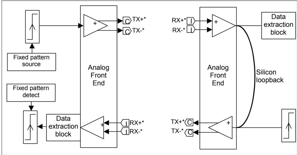
**Figure 40 – Loopback far-end analog**
