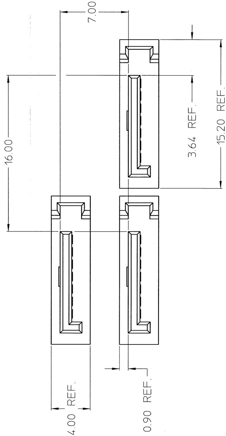
Figure 13 – Recommended host plug connector clearance or spacing
