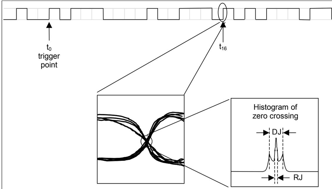
**Figure 43 – Jitter measurement example**
