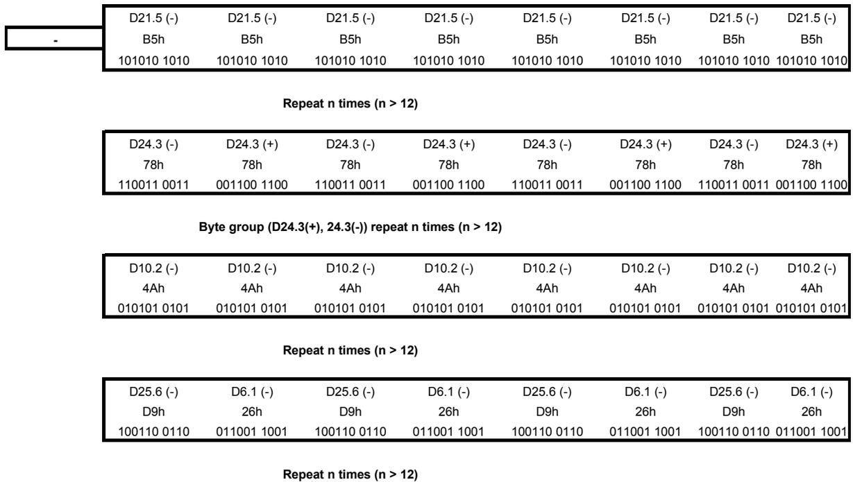
**Figure 35 - Half-rate / quarter-rate high transition density pattern**
