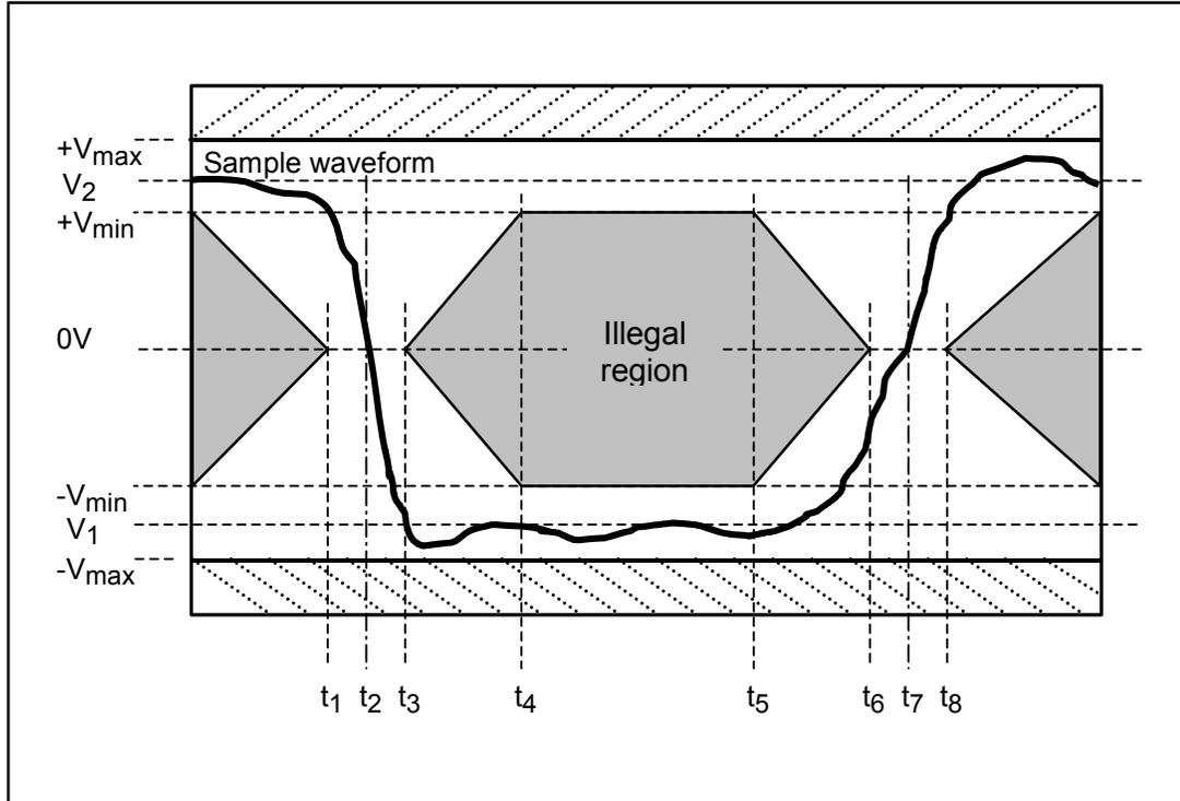
Figure 21 – Voltage / timing margin base diagram
