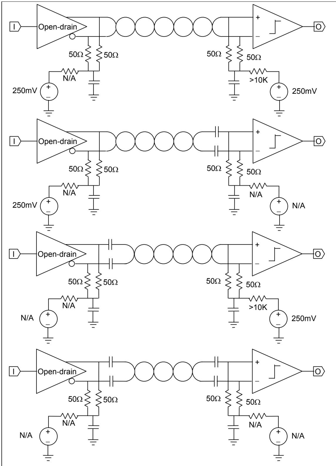
Figure 27 – Common-mode biasing
