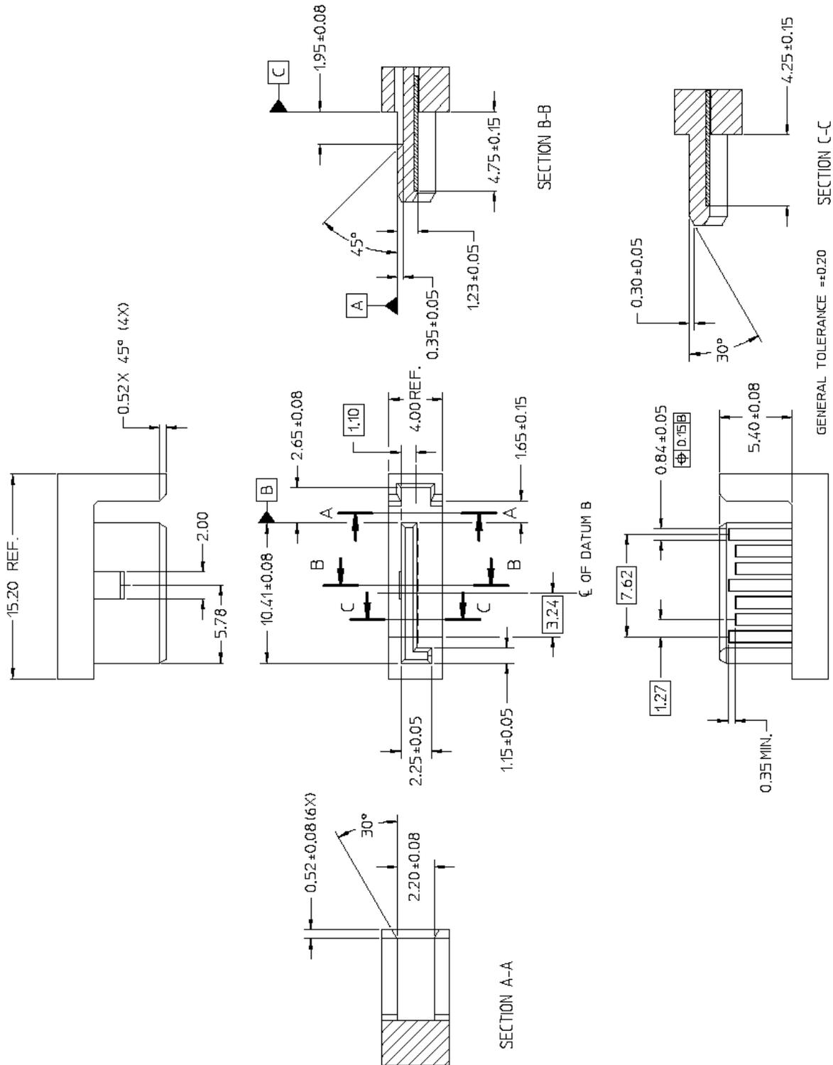
Figure 12 – Host plug connector interface dimension
