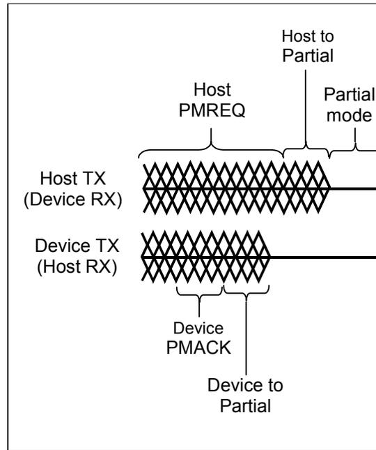
Figure 48 – On to Partial/Slumber - host initiated
