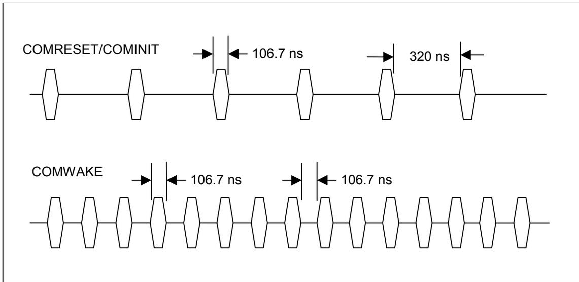
**Figure 28 – Out of band signals**
