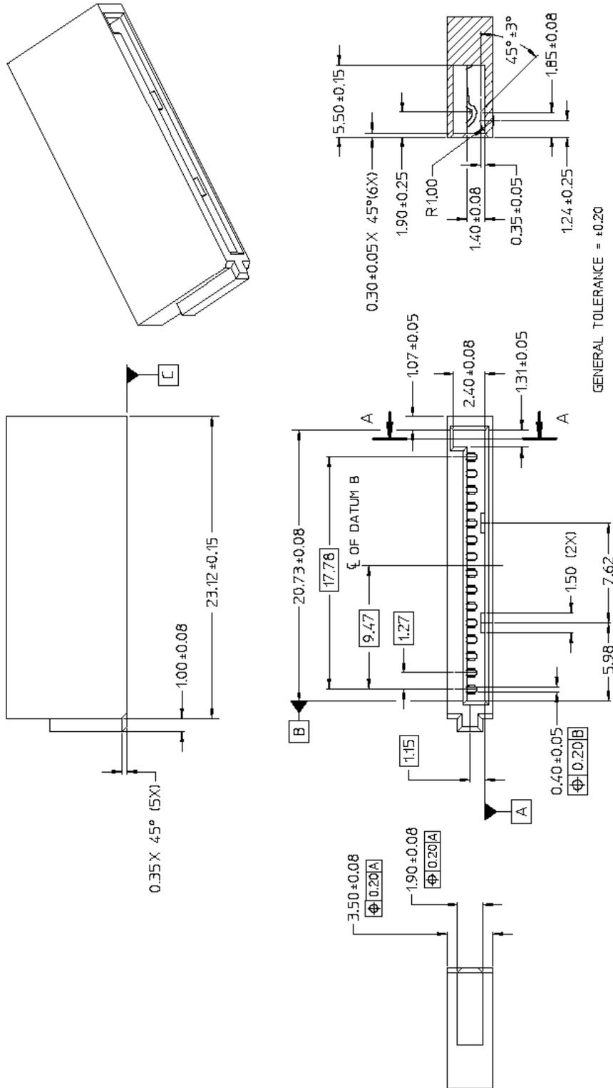
Figure 15 – Power receptacle connector interface dimensions
