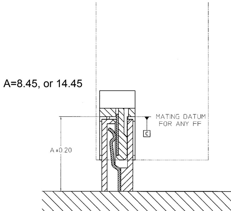
**Figure 17 - Device-backplane mating configuration**
