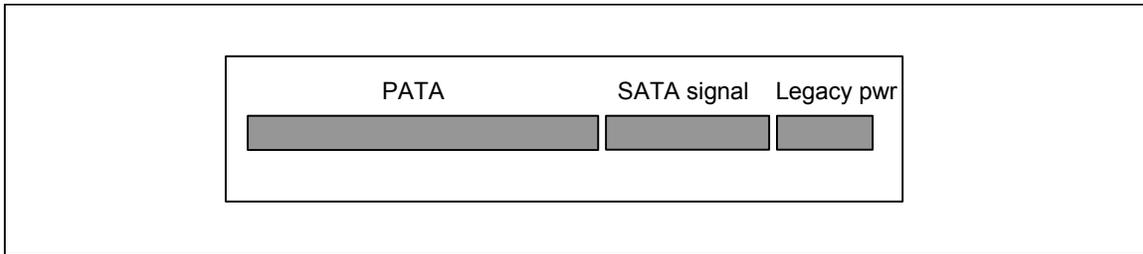
**Figure 74 - Device connector configuration 35C1**
