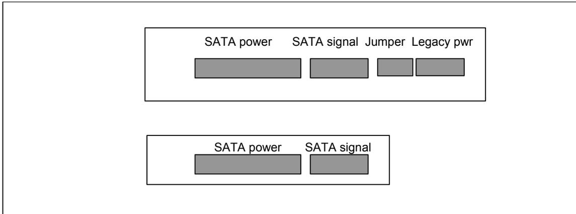
The reference connector configuration for the 3.5" device includes the Serial ATA connector with both signal and power segments, and the legacy jumper and power connectors for smooth transition from Parallel ATA.
