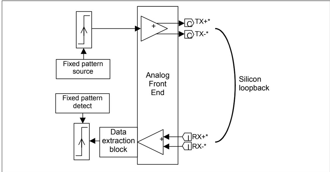
**Figure 41 – Loopback - near-end analog**
