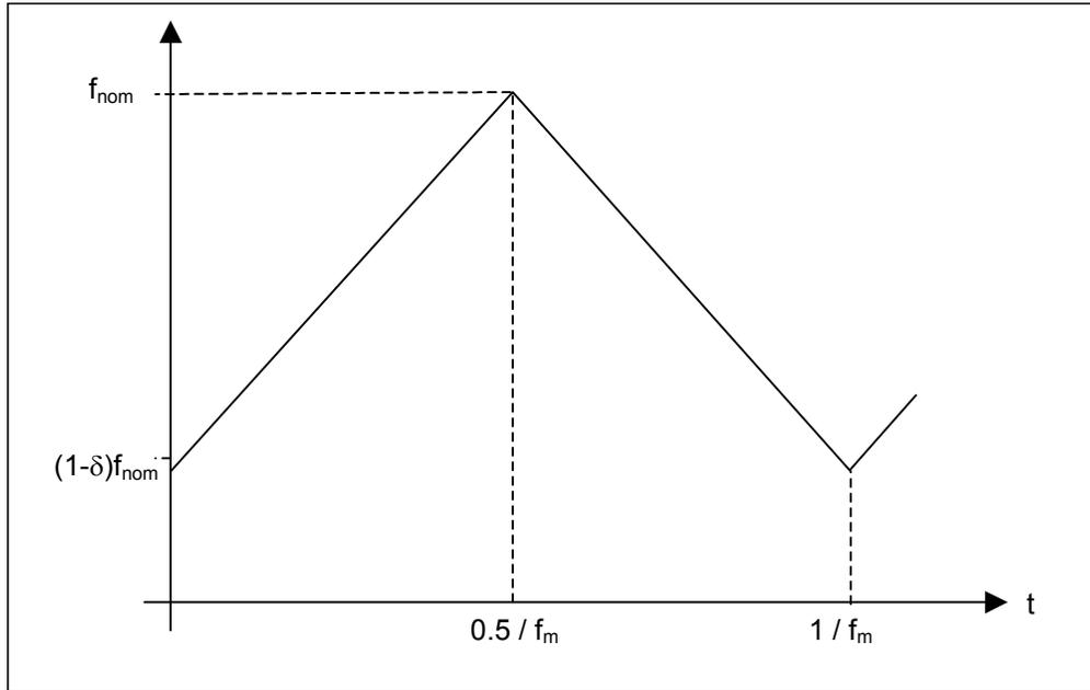
**Figure 25 - Triangular frequency modulation profile**
