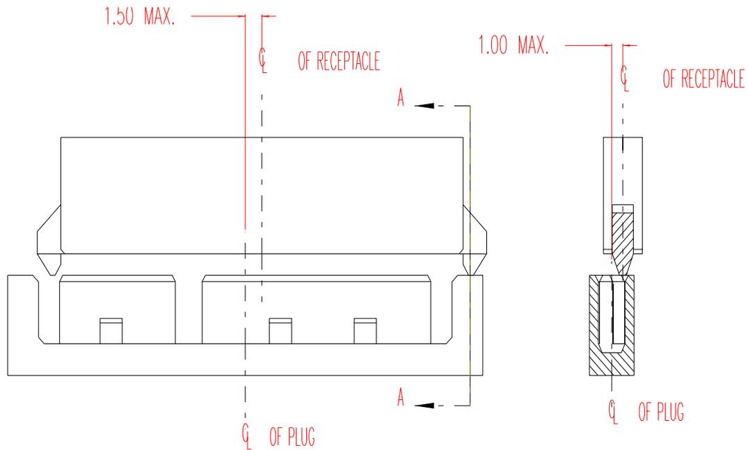
**Figure 16 – Connector pair blind-mate misalignment tolerance**
