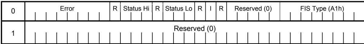
**Figure 61 - Set Device Bit - Device to Host FIS layout**
