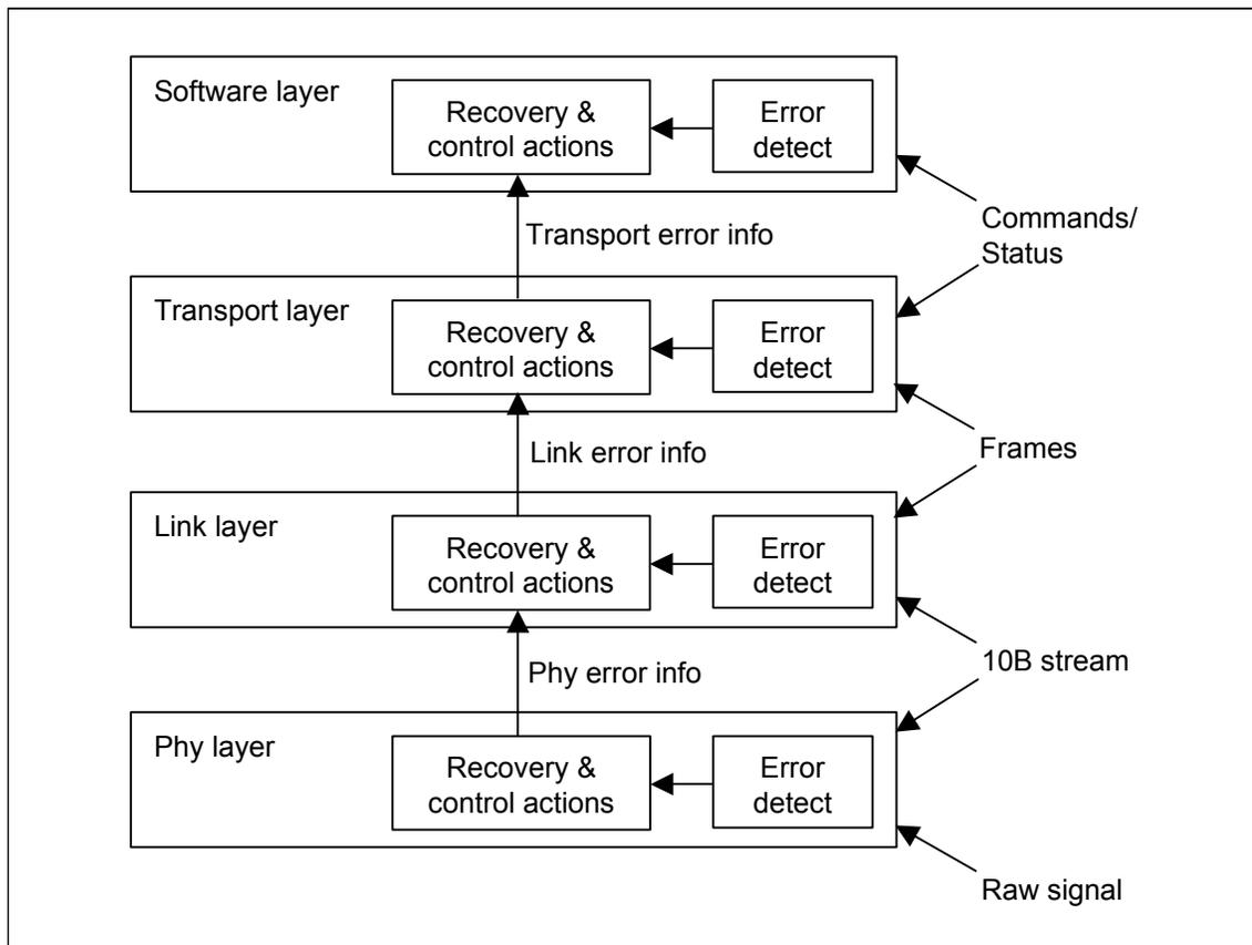
Figure 67 – Error handling architecture
