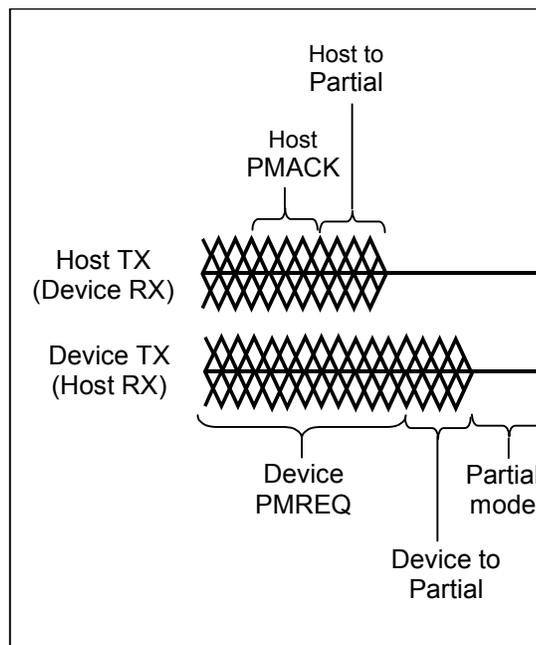
Figure 49 – ON to Partial/Slumber - device initiated
