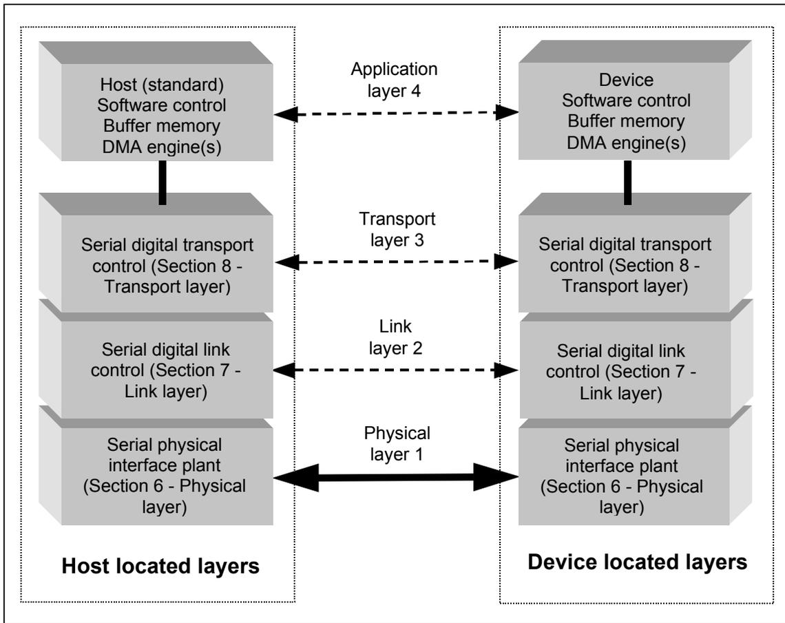
Figure 4 – Communication layers
