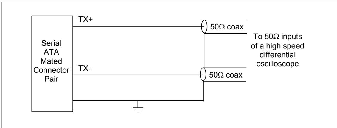
**Figure 45 – Transmit test fixture**
