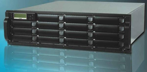
SCSI U320 / FC to SATA Subsystems Powered with Enhanced RAID 6 and S.M.A.R.T Technology - Supreme Data Protection for Mission Critical Application
