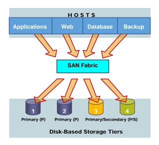
In the above conceptual diagram, we see the range of hosts, inclusive of any top-level applications, databases, web servers, and backup/restore servers, all connected to a SAN fabric. Within this SAN, the disk storage targets are classified within usage tiers numbered from 1 to 4. We define these classes as follows:
