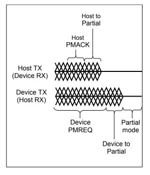
Figure 49 – ON to Partial/Slumber - device initiated
