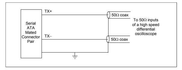
Figure 45 – Transmit test fixture
