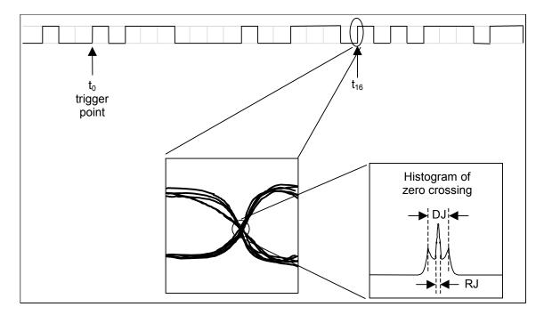
Figure 43 – Jitter measurement example
