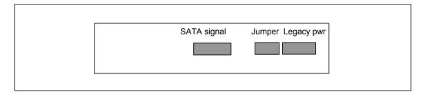
Figure 70 - Device connector configuration 35B2
