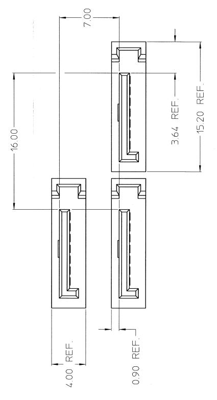
Figure 13 – Recommended host plug connector clearance or spacing
