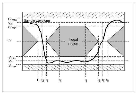
Figure 21 – Voltage / timing margin base diagram
