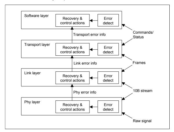
Figure 67 – Error handling architecture
