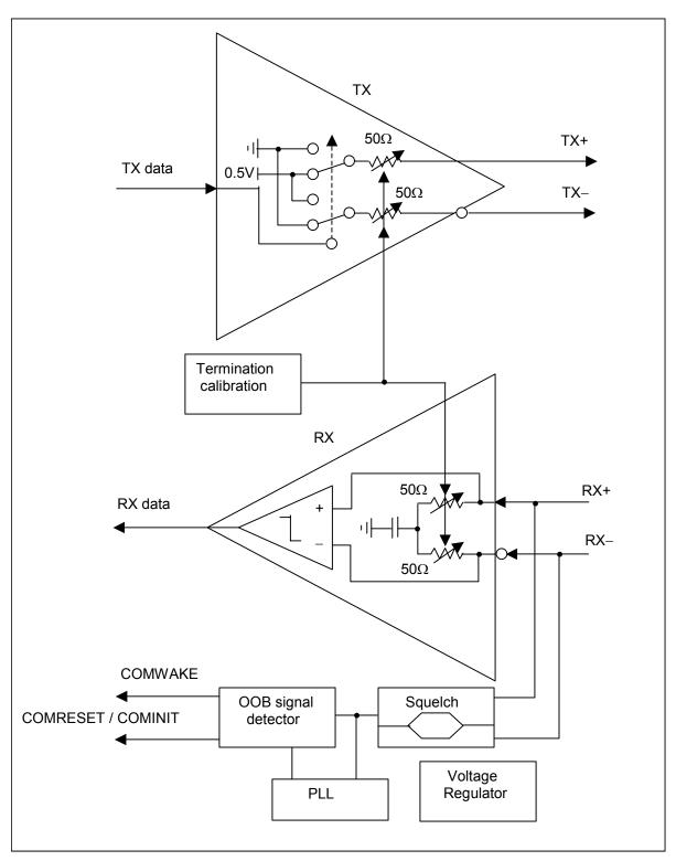
Figure 19 – Analog front end (AFE) block diagram
