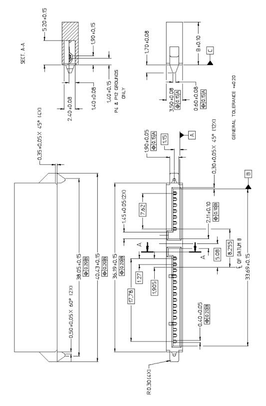
Figure 14 – Host receptacle connector interface dimensions
