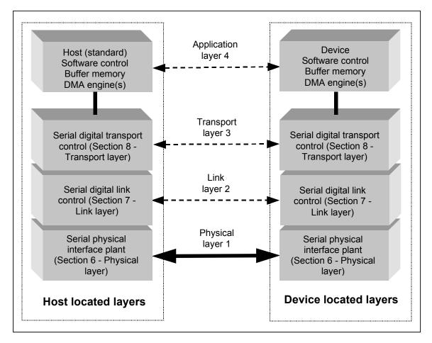
Figure 4 – Communication layers
