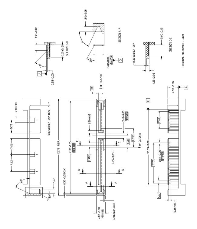
Figure 9 – Device plug connector interface dimensions
