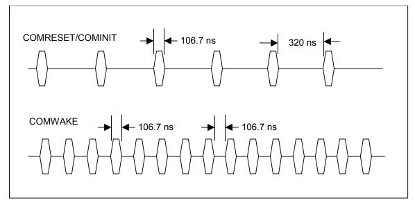
Figure 28 – Out of band signals
