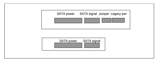
The reference connector configuration for the 3.5" device includes the Serial ATA connector with both signal and power segments, and the legacy jumper and power connectors for smooth transition from Parallel ATA.
