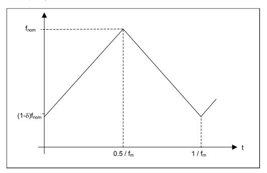
Figure 25 - Triangular frequency modulation profile
