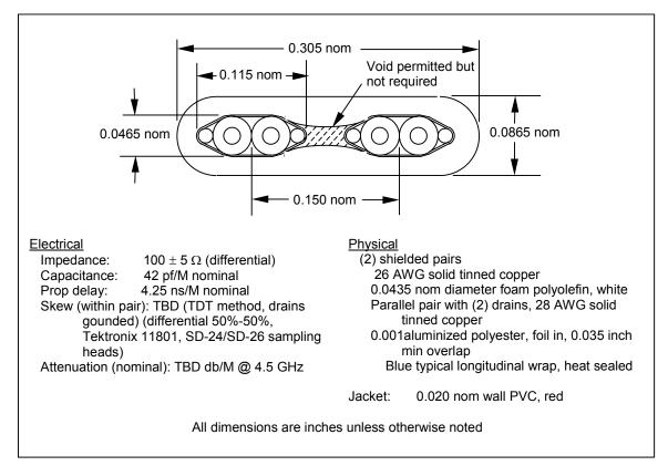
Figure 76 – Cable construction example
