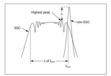
Figure 26 - Spectral fundamental frequency comparison
