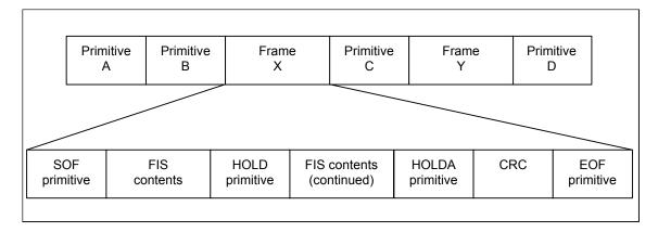
Figure 57 – Transmission structures
