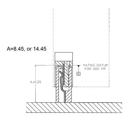
Figure 17 - Device-backplane mating configuration
