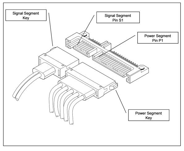
Figure 10 Connector Pin and Feature Locations
