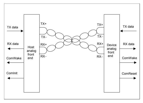
Figure 20 – Analog front end (AFE) cabling
