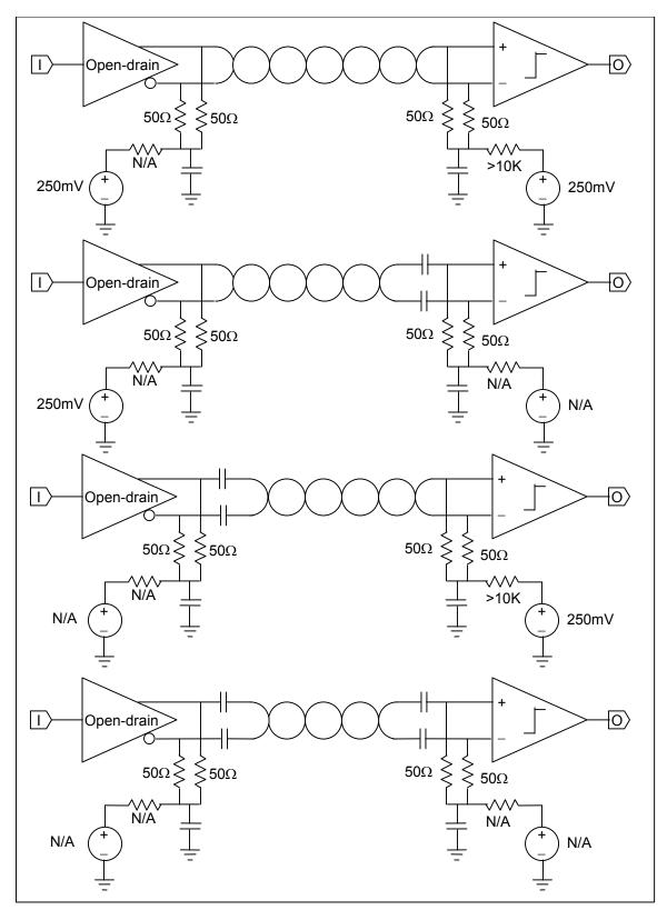
Figure 27 – Common-mode biasing
