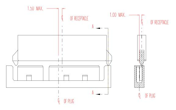
Figure 16 – Connector pair blind-mate misalignment tolerance
