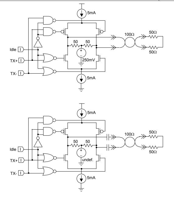
Figure 29 – Transmitter examples (concluded)
