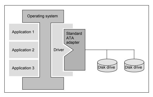
Figure 2 – Standard ATA device connectivity
