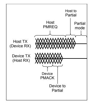
Figure 48 – On to Partial/Slumber - host initiated
