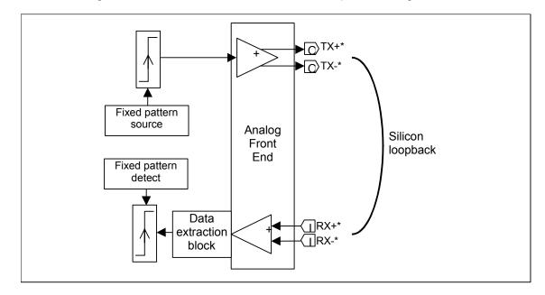
Figure 41 – Loopback - near-end analog
