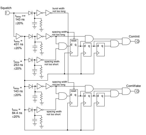
Figure 32 – OOB signal detector
