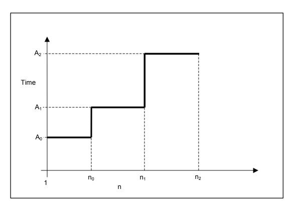
Figure 22 – Jitter output/tolerance mask
