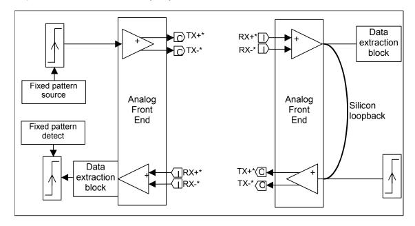
Figure 40 – Loopback far-end analog
